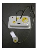
**Electronic Control**. Students construct a thyristor based latching circuit and explore the possible applications for such circuits. A wide range of input and output devices are introduced and students then go on to design and manufacture an alarm circuit of their own choice and fit it in a custom housing.
